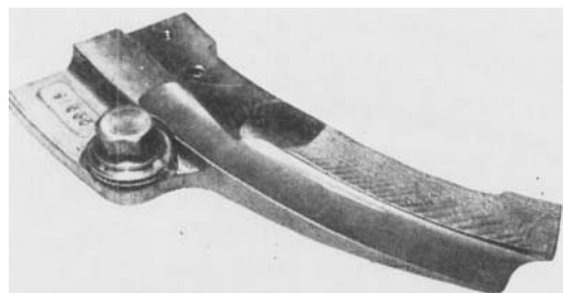
Fig. 3—Photograph of ejection track and force washer.
